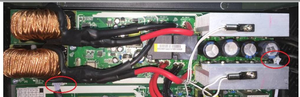
Remove the screws on the MPPT board.
