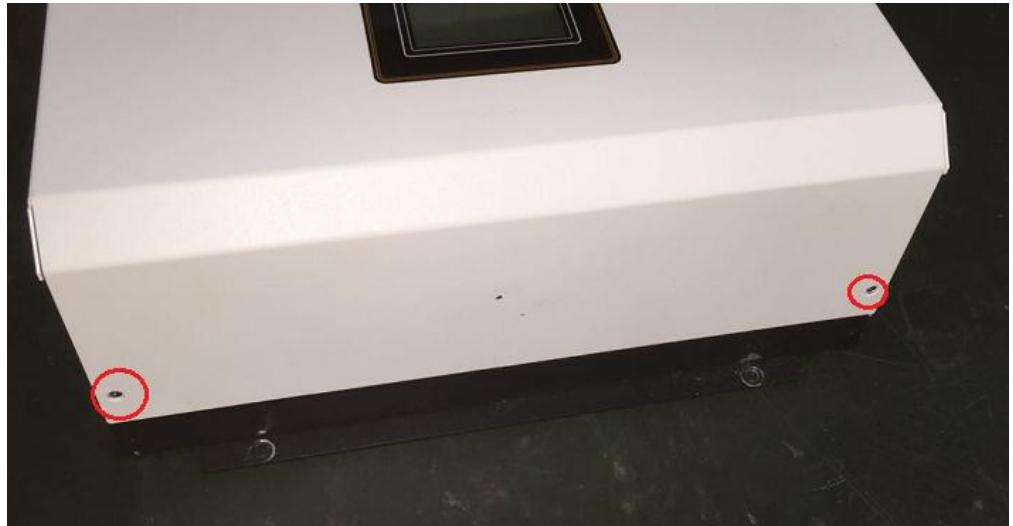
Open the top cover carefully, for there are two cables connected with LCD display.
